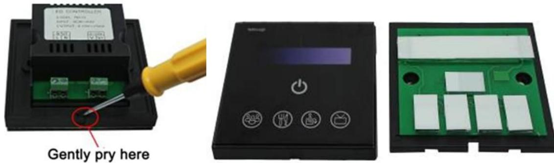
2、 The controller is fixed on the wall bottom shell with 86 × 86 installation box screws (box installed customers need to purchase their own), as shown below:
