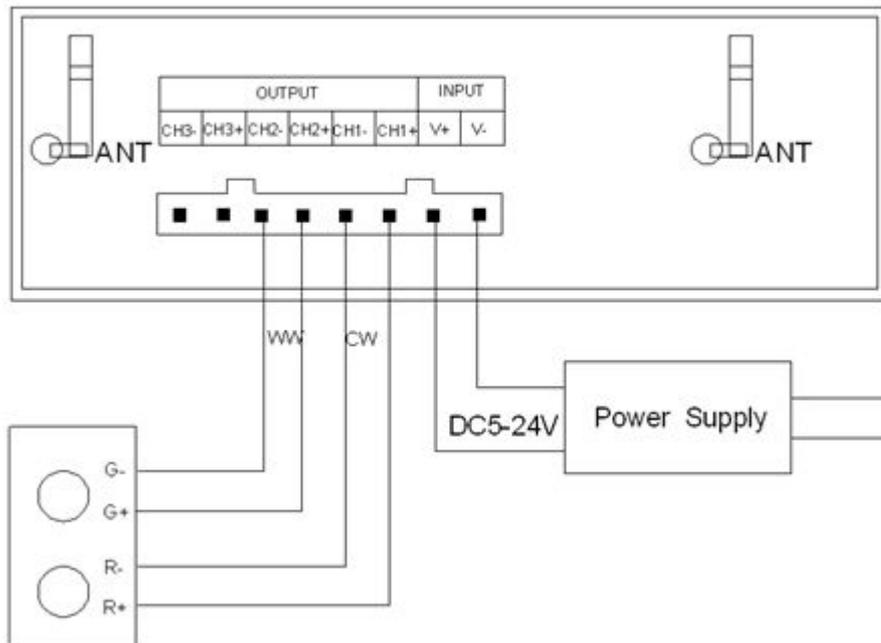
When connect three channels LED, you should put the Dream Color software switch to CD mode to use,only under this mode,you can control the LED's color temperature,brightness and color temperature shortcut key settings.Color disk adjust the color temperature(meanwhile top left CW,WW numerical with change),brightness item adjust bright,"M"key set the special color temperature state.
