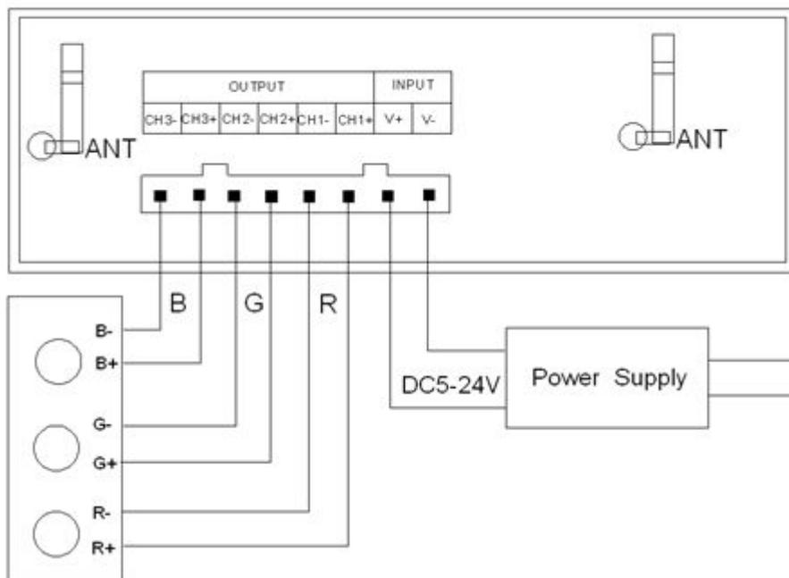
When connect three channels LED, you should put the Dream Color software switch to CD mode to use, only under this mode, you can control the LED's color, brightness and speed. Color disk adjust the
