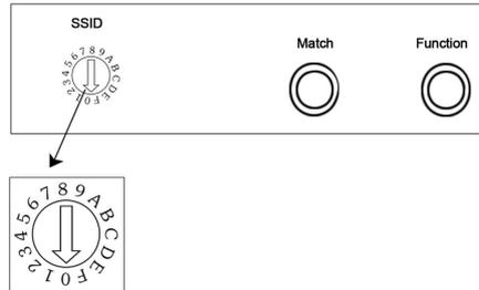
The dial code is used for setting LED-WiFi controller Ssid number, corresponding table as below. Form 0 to 15, have 16 code in total, so our Ssid number fasten to LN001 to LN016. That means use our product in same small area can set 16 mutual isolation LAN, once the dial code changed after switch was dialed, Ssid number immediately be modified, so you need to note that it need to search and connect again.
