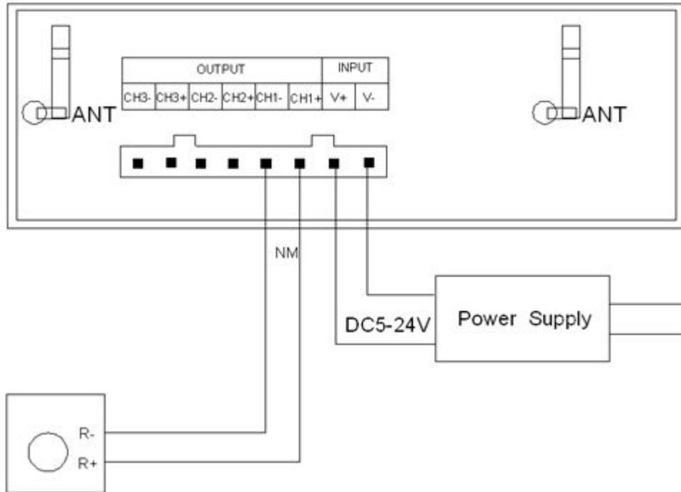
When connect three channels LED, you should put the Dream Color software switch to CD mode to use, under this mode, use color disk control the LED's brightness, Adjust process can be seen in the upper left corner NM numerical with change.
