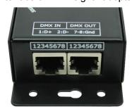
**DMX IN**: input interface of DMX signal, D+ should be connected with positive of signal, D- connected with negative of signal, Gnd connected with ground.
