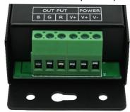
**POWER**: input interface of power, V+ should be connected with positive of power, V- connected with negative of power, the range of supply voltage is DC5-24V
