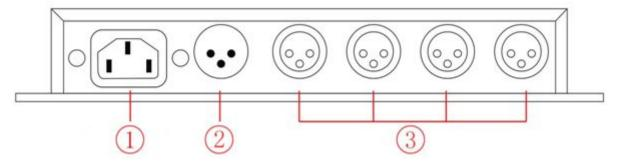
(1) AC100-240V power interface @DMX signal input interface @DMX signal output interface
