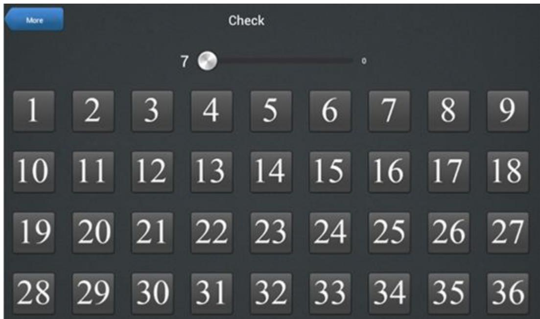
Number 1 to 36 responds to 36 channel, you can choose every channel, after that, sliding the bar to test if each channel is connected well.
