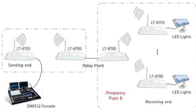
5.3 Extend the communication distance by boost antenna:
