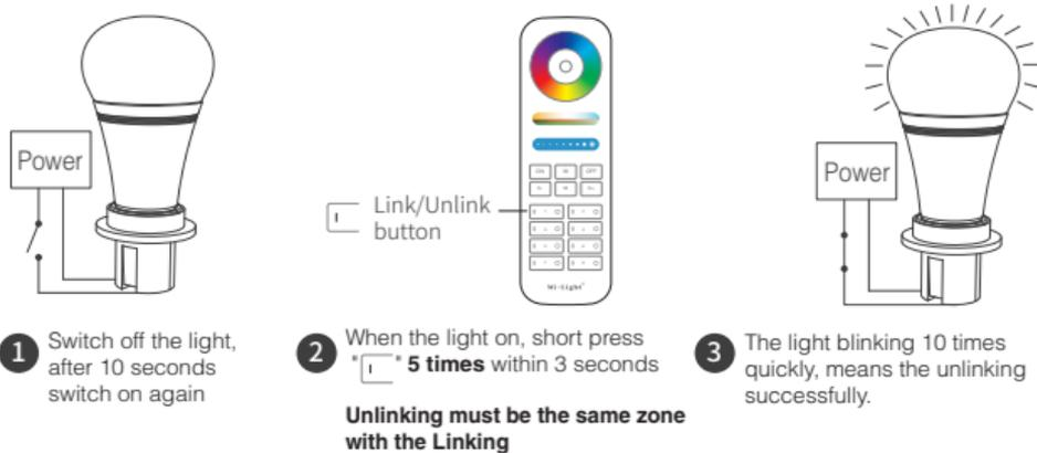
**!** If the light not blink quickly, the unlink failed, pls switch off the light again, and follow the above steps to unlink again.
