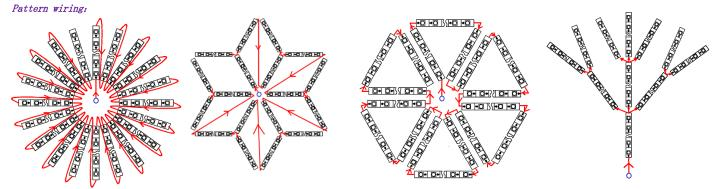
In the figure, the red line is the signal line. Since the impedance of the joint is indefinite, it is necessary to connect the power supply from the equal parts of the pattern to ensure that the power supply is balanced everywhere and the brightness and color are consistent everywhere.
