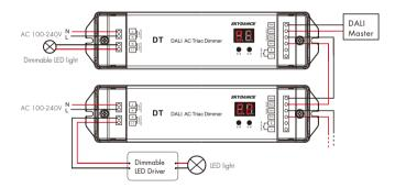
Please carefully ensure all wire connections and polarities are correct and securbefore applying power otherwise this controller will be damaged.
