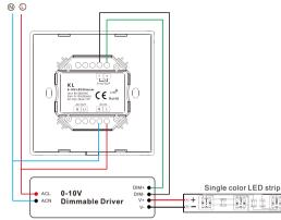
• KL connect with 0/1-10V dimming driver (use AC OUT)
