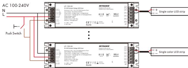
The provided AC Push-Dim interface allows for a simple dimming method using commercially available non-latching (momentary) wall switches.
