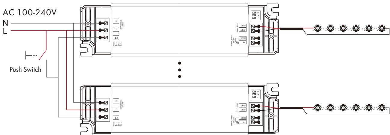
The provided AC Push-Dim interface allows for a simple dimming method using commercially available non-latching (momentary) wall switches.
