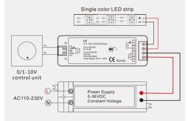
LED power supply voltage and power select : 5V lamp, Input 5V power supply, can load 0~40W, 12V lamp, Input 12V power supply, can load 0~96W, 24V lamp, Input 24V power supply, can load 0~192W, 36V lamp, Input 36V power supply, can load 0~288W, The power supply power must larger than load power 20%.
