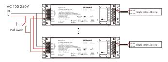
The provided AC Push-Dim interface allows for a simple dimming method using commercially available non-latching (momentary) wall switchs.
