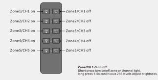
R1-1 is default as 5 zone dimming remoter, also can be used as single zone 5 channel dimming remoter. 1 ON + 5 ON: Long press 2s set as 5 channel dimming remoter, match with one receiver of 5 channel,
