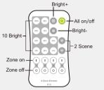
All on/off: Turn on/off all 4 zone light. 1,2,3,4 zone on/off: Turn on/off zone light. at the same time, select current zone. Continuous short press multiple zone on key, can synchronous select multiple zone. Bright+/-: Adjust brightness for current selected zone, short press 10 levels.
