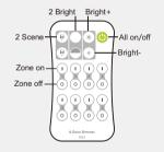
All on/off: Turn on/off all 8 zone light. 1,2,3,4,5,6,7,8 zone on/off: Turn on/off zone light, at the same time, select current zone. Continuous short press multiple zone on key, can synchronous select multiple zone. Bright+/-: Adjust brightness for current selected zone, short press 10 levels, long press 1-5s continuous 256 levels adjustment. 2 Scene: Short press run the scene, long press 2s save. 8 zone run or save synchronously.
