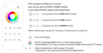
: For RGB+CCT(WW/NW) lamp, adjust color temperature by WW/NW channel, short press 11 levels, long press 2s get max or min color temperature.
