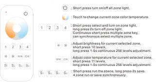
Each zone also can match single color controller or lamp. At this time, touch wheel will adjust brightness.
