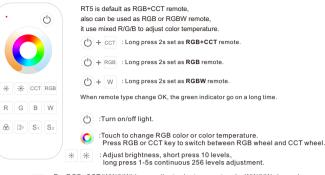
CCT : For RGB+CCT(WW/NW) lamp, adjust color temperature by WW/NW channel, short press 11 levels. long press 2s get max or min color temperature.
