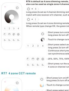
also can be used as single zone 4 channel dimming remote. Long press 2s set as 4 channel dimming remote. match with one receiver of 4 channel, such as V4 or C4 controller. Long press 2s set as 4 zone dimming remote, match with four dimming receivers. When remote type change OK, the green indicator go on a long time. : Short press turn on/off current zone light, long press 2s turn off all zone light : Touch to change current zone brightness.
