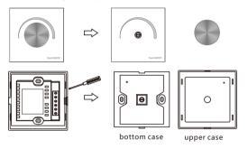
2. After connect wires, put bottom case into 86 bottom box, put in the screw and tighten.
