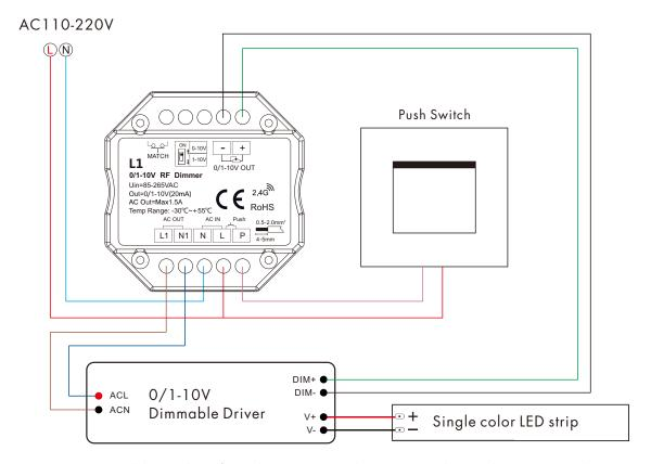
**Note:** We recommend the number of LED drivers connected to 0/1-10V dimmer does not exceed 5 pieces, The maximum length of the wires from dimmer to LED driver should be no more than 15 meters.
