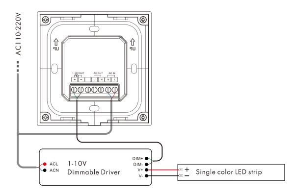
• Connect with 1-10V dimming driver (use AC OUT)
