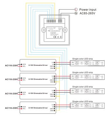
T18 have same wiring diagram, just only connect with one 0-10V dimming driver,
