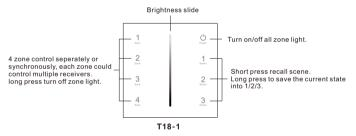
Note: After touch power key to turn off light, long press power key for 5 seconds will turn on or turn off tone.
