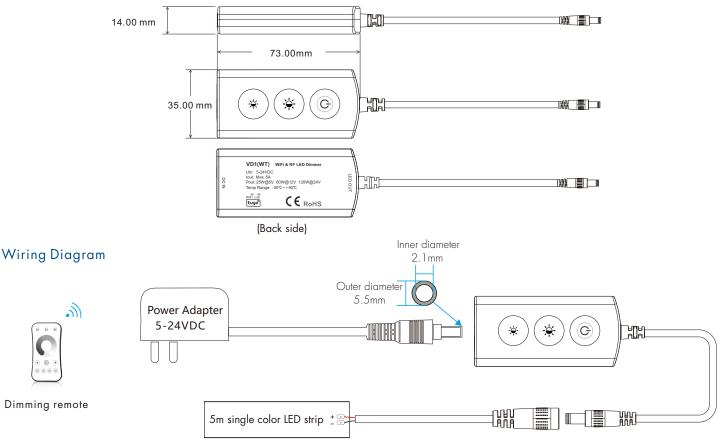
Note: Press and hold the (③) and (\*) (Brightness-) button for 2s, output LED flashes 3 times, the light on/off fade time will change between 3s and 0.5s.
