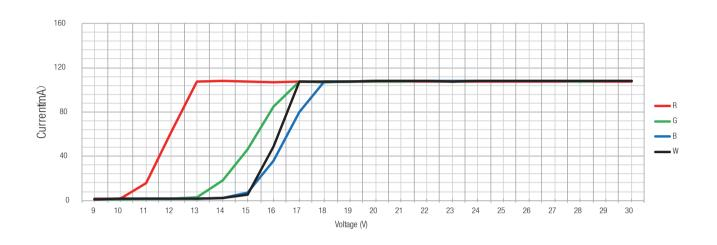
Note: This curve is tested when the IP20 1M LED Strip is under thermal stability after 2hrs continuous working in 15 °C room temperature.
