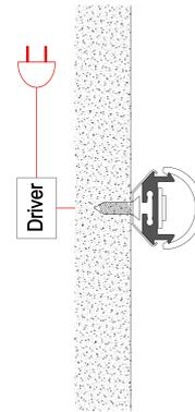
**The second option:** 1. Mount the LED strip(D), insert the cover(E), insert the end
