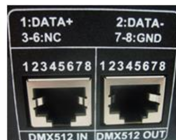
DMX input/output interface: RJ45 Interface
