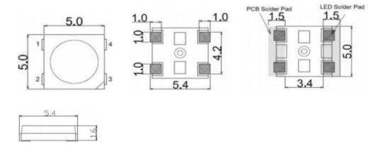
Notes: All dimensions are in millimeters; if not otherwise noted, tolerance ranges of ±0.2mm are normally used.
