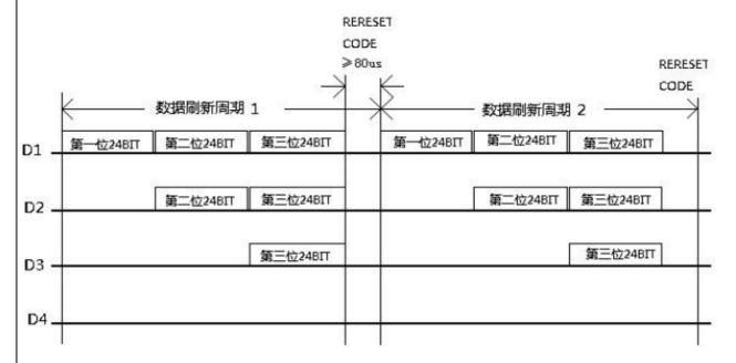
Note: D1 is the data sent from the MCU side, and D2, D3 and D4 are the data automatically shaped and forwarded by the cascade circuit.
