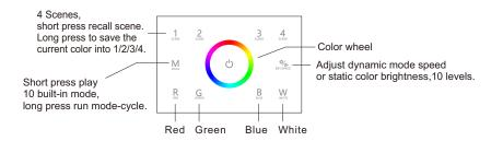
Note: After touch power key to turn off light, long press power key for 5 seconds will turn on or turn off tone.
