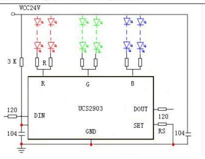
In order to prevent the damage of charged pull plug, when 24 v power supply, Din and Do all the string in a 120 ohm resistor for protection
