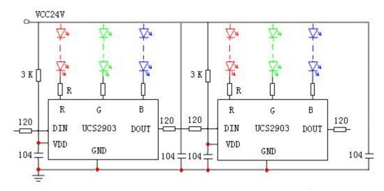
In order to prevent the damage of charged pull plug, when 24 v power supply, Din and Do all the string in a 120 ohm resistor for protection
