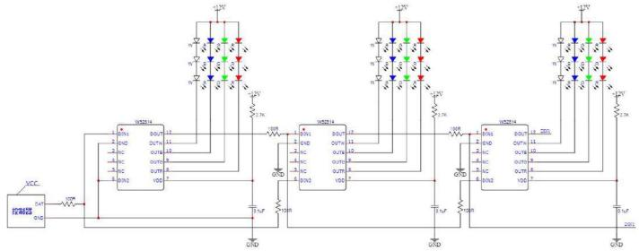
2. Supply voltage=24V(Each channel drives 6LEDs)
