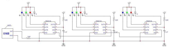
2. Supply voltage=12V (Each channel drives 3 LEDs)
