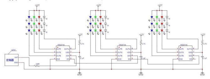
3. Supply voltage=24V (Each channel drives 6 LEDs)
