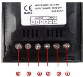
① GND ② VCC Input ③ VCC Output ④ R Output ⑤ G Output ⑥ B Output
