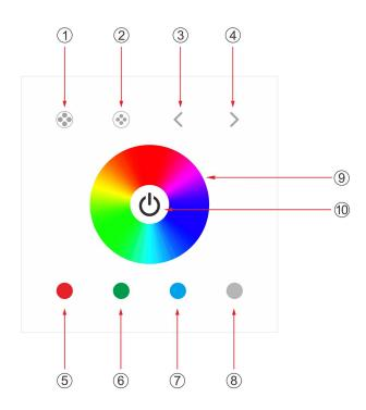
①:mode increase—when the controller is open, mode can be increased(the highest is 21)
