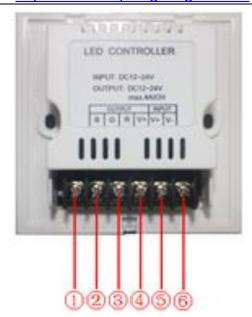
①: blue light cathode; ② green light cathode; ③ red light cathode; ④common anode; ⑤input power anode; ⑥input power cathode。
