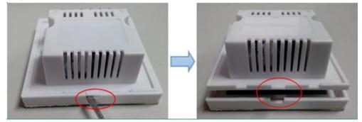
7.1.2 remove the cable. Pull the locking of the wiring seat, and then you can slowly remove the cable, as shown below:
