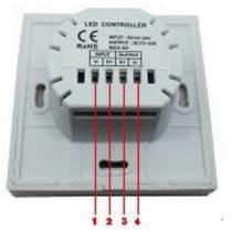
"1"、 "2": power input pins, input voltage range is 12-24V, "1" is negative, "2" is positive; "3"、 "4": power output pins, output voltage is 12-24V, output maximum current is 8A, "3" is positive, "4" is negative.
