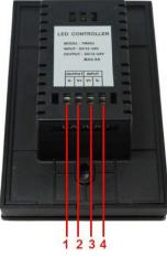
3 and 4: power input, input voltage range: 12-24V, 3 for positive, 4 for negative.
