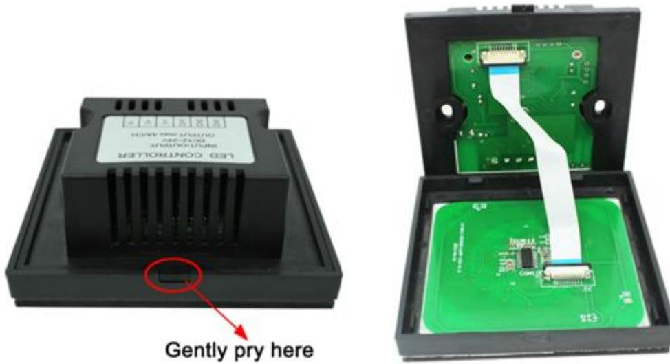
(2) remove the cable. Pull the locking of the terminal transposon, and then you can slowly remove the cable, as shown below:
