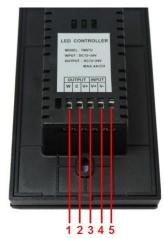
4 and 5: power input, input voltage range: 12-24V, 4 for positive, 5 for negative.
