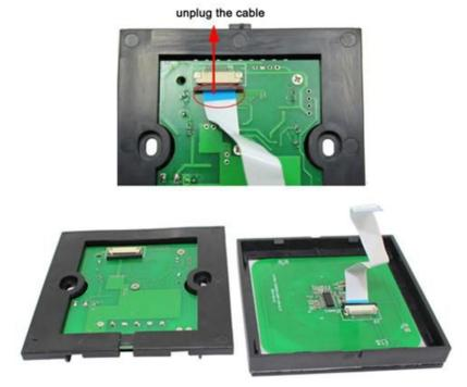
3. Fix the base of controller in the  $86 \times 86$  installation box (customers need to buy the installation box by themselves) on the wall with screws.
