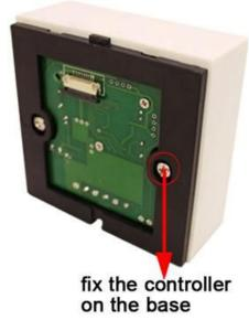
(4) use your hand gently pull down the cable seat lock according to step 2, plug the cable into cable seat, press the lock, and mount the cable of panel on the base, as shown below:
