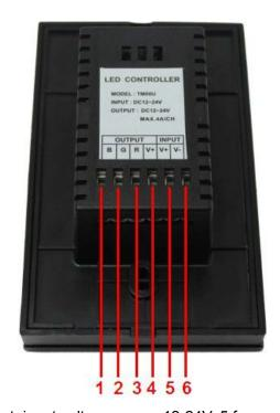
5 and 6: power input, input voltage range: 12-24V, 5 for positive, 6 for negative.
