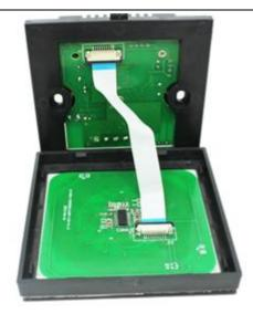
(2) remove the cable. Pull the locking of the terminal transposon, and then you can slowly remove the cable, as shown below:
