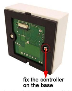
(4) use your hand gently pull down the cable seat lock according to step 2, plug the cable into cable seat, press
