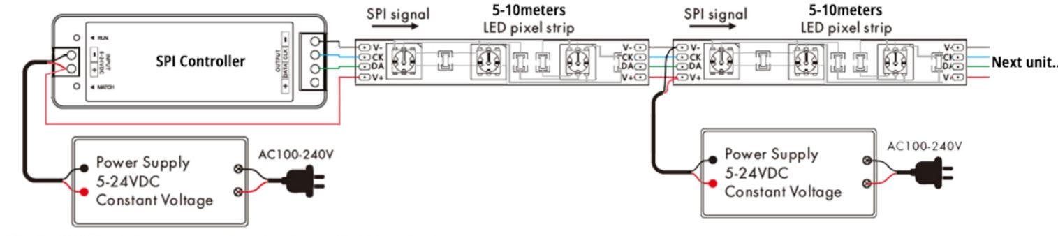
Note: the total pixels should be lower than the output pixels of the controller
